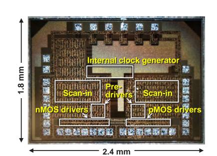
Hybrid DC-DC converters for automotive applications (Mixed inductors and capacitors reduce losses.)
