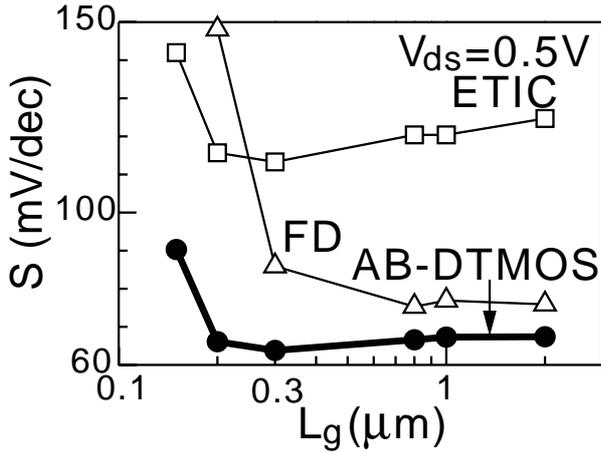
Fig. 5. Dependence of subthreshold slope on gate length. AB-DTMOS has an ideal subthreshold slope and suppresses the short channel effect well.
