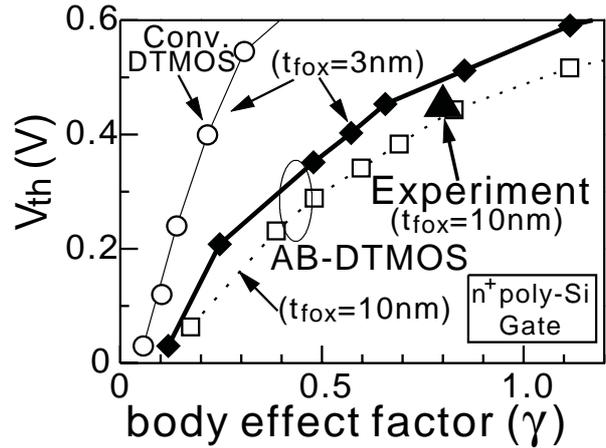
Fig. 7. Dependence of  $V_{th}$  on  $\gamma$  by the simulations for the conventional DTMOS (gate oxide thickness is 3 nm), and AB-DTMOS (gate oxide thickness is 3 nm or 10 nm). In the conventional DTMOS, a uniformly doped channel profile is assumed. Experimental data ( $V_{th} = 0.45$  V,  $\gamma = 0.8$ ) is also plotted.  $\gamma$  of AB-DTMOS is twice as large as that of the conventional DTMOS at a fixed  $V_{th}$ .
