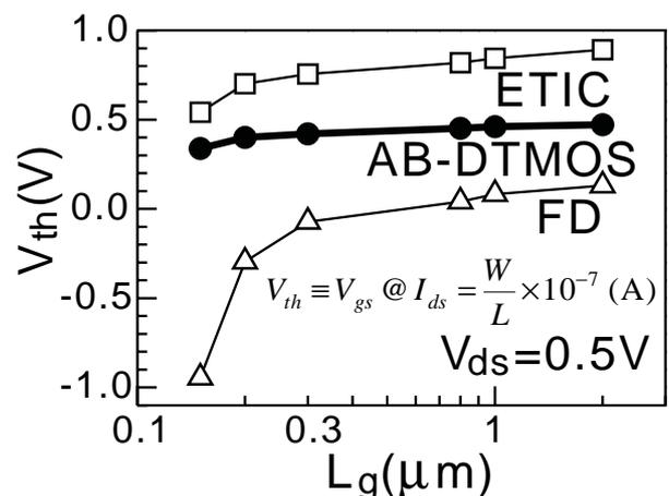
Fig. 4. Dependence of  $V_{th}$  on gate length. AB-DTMOS has appropriate  $V_{th}$  and suppresses the short channel effect well. The definition of  $V_{th}$  is shown in the inset.
