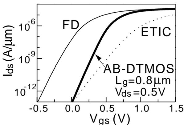
Fig. 2. Subthreshold characteristics of the FD SOI MOSFET, ETIC-SOI MOSFET, and AB-DTMOS shown in Table I. The gate length is  $0.8 \mu\text{m}$ .
