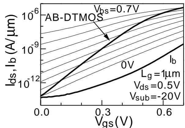
Fig. 3. Subthreshold characteristics of AB-DTMOS and ETIC-SOI MOSFET where body voltage ( $V_{bs}$ ) is varied from 0 V to 0.7 V by 0.1 V steps. Body current ( $I_b$ ) of AB-DTMOS is also shown. Derived  $\gamma$  is as high as 0.8.
