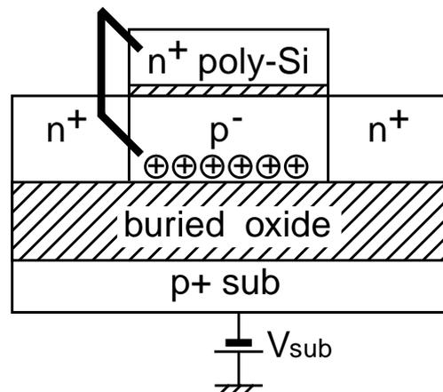
Fig. 1. A schematic view of AB-DTMOS. The back interface between the non-doped thin SOI and the buried oxide is accumulated by a large negative substrate bias. The gate electrode is connected to this electrically induced body.
