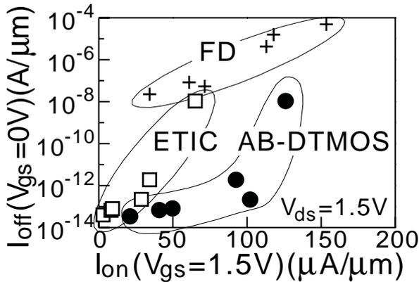
Fig. 6. On/off characteristics of FD SOI MOSFET, ETIC-SOI MOSFET, and AB-DTMOS. The gate length is varied. AB-DTMOS shows a high current drive and a low off-current. However, ETIC-SOI MOSFET shows a low current drive and FD SOI MOSFET shows a high off-current.
