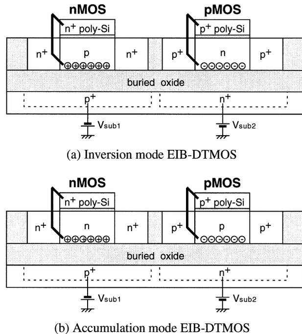
**Fig. 10** Schematic cross-sections of EIB-DTMOS. Inversion mode EIB-DTMOS and accumulation mode EIB-DTMOS are shown. Different substrate biases,  $V_{sub1}$  and  $V_{sub2}$ , are applied to NMOS and PMOS, respectively.  $V_{sub1}$  and  $V_{sub2}$  are supplied from the front via contact holes through the buried oxide.
