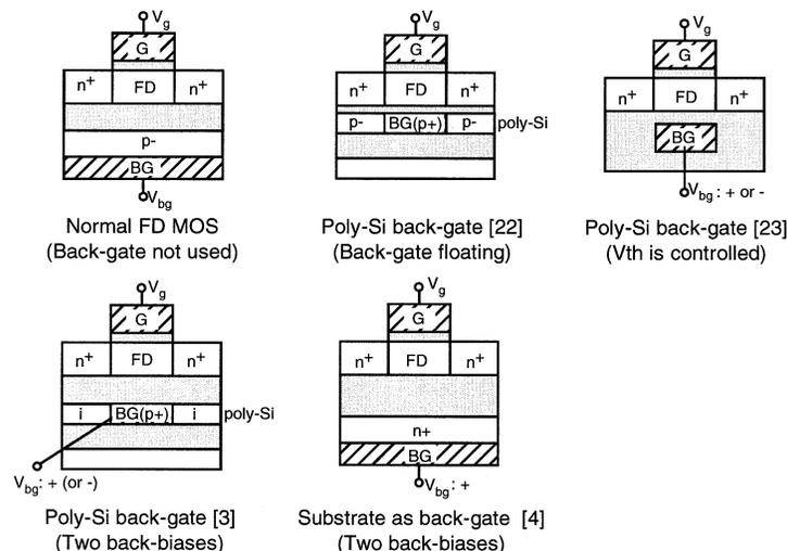
**Fig. 5** Schematic cross-sections of examples of FD SOI MOSFETs. Normal FD SOI MOSFET and some other structures with buried back-gates are shown.
