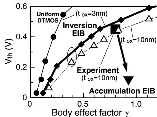
**Fig. 11** Relation between body effect factor and threshold voltage obtained by simulation in DTMOS. Uniformly doped DTMOS and an inversion mode EIB-DTMOS with a slightly B-doped body region are shown. An experimental datum is plotted. An accumulation mode EIB-DTMOS is also plotted.
