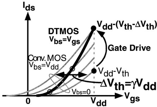
Fig. 8 Schematic characteristics of DTMOS.
