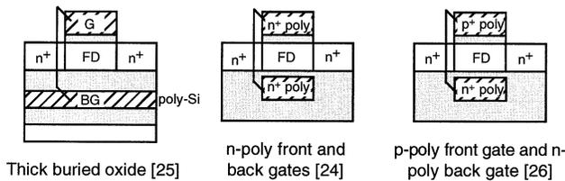
Fig. 6 Schematic cross-sections of examples of DG MOSFETs.
