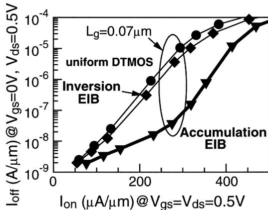
**Fig. 12** Relation between current drive and off-current in uniformly doped DTMOs, inversion mode DTMOs, and accumulation mode DTMOs. Threshold voltage is fixed at  $L_g = 0.5 \mu\text{m}$ , and  $L_g$  is varied. Gate oxide thickness is 3 nm and junction depth is 15 nm.
