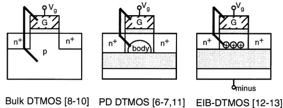
**Fig. 4** Schematic cross-sections of variations of DTMOS. Bulk DTMOS, PD DTMOS, and EIB-DTMOS are shown.
