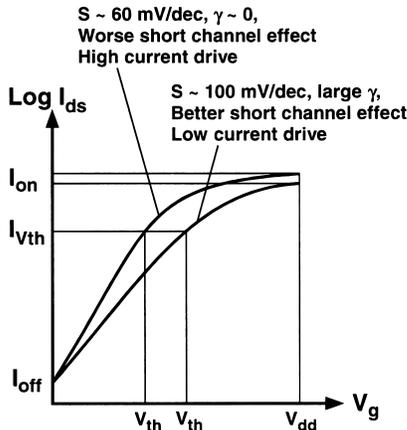
**Fig. 1** A schematic illustration of the relationships among the subthreshold swing, body effect factor, short channel effect, and current drive.
