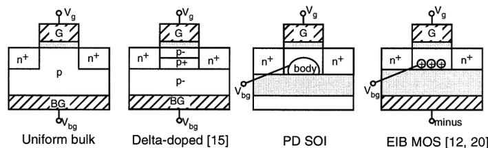
**Fig. 3** Schematic cross-sections of variations of “conventional MOS.” Uniformly doped bulk MOSFET, delta-doped MOSFET, PD SOI MOSFET, and EIB MOSFET are shown.
