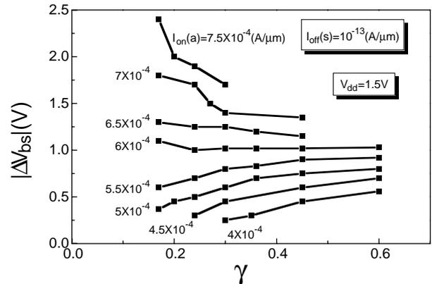
Fig. 6. Contour lines of  $I_{\text{on}}(\text{a})$  in a VT MOS as a function of  $|\Delta V_{\text{bs}}|$  and  $\gamma$ . The  $V_{\text{dd}}$  is 1.5 V. When  $|\Delta V_{\text{bs}}|$  is larger than 1.2 V, a higher  $I_{\text{on}}(\text{a})$  is obtained for larger  $\gamma$ . On the other hand, when  $|\Delta V_{\text{bs}}|$  is less than 1.2 V, higher  $I_{\text{on}}(\text{a})$  is obtained for smaller  $\gamma$ .
