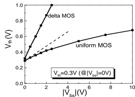
Fig. 9. Relation between  $V_{th}$  and  $|V_{bs}|$ . In a uniform MOS,  $\Delta V_{th}$  is proportional to the square root of  $V_{bs}$ . In delta MOS,  $\Delta V_{th}$  is almost proportional to  $V_{bs}$ . Channel profile should be as steep as in the delta MOS, and a super steep channel profile is strongly desired in scaled VTMS.
