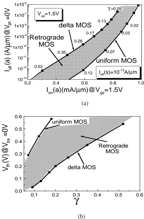
Fig. 3. (a) Relation between  $I_{off}(a)$  and  $I_{on}(a)$  in a uniform MOS and delta MOS.  $I_{off}(s)$  of each device is fixed at  $10^{-13}\text{A}/\mu\text{m}$ . The value of  $\gamma$  each device are shown. (b) Relation between  $V_{th}$  and  $\gamma$  in a uniform MOS and delta MOS. The channel-engineered MOSFETs, such as retrograde MOS, cover the area between the two lines.  $|V_{bs}|$  and  $\gamma$  cannot be varied widely by using only uniform, retrograde or delta MOS.
