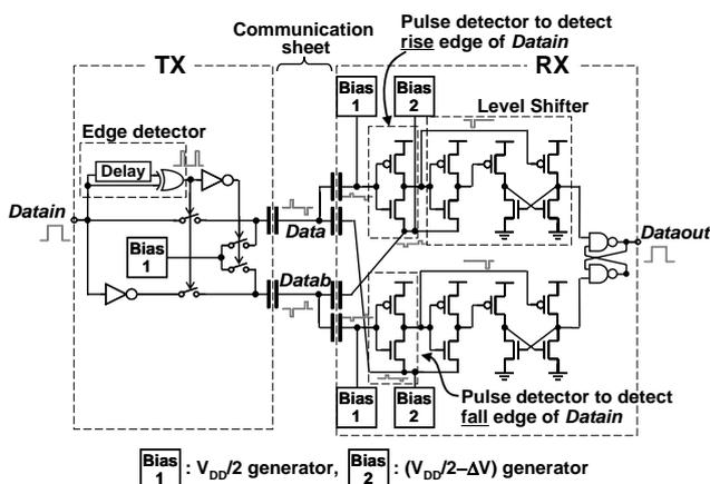
Fig. 3 Schematic of transceiver with data edge signaling and DC power-free pulse detector.
