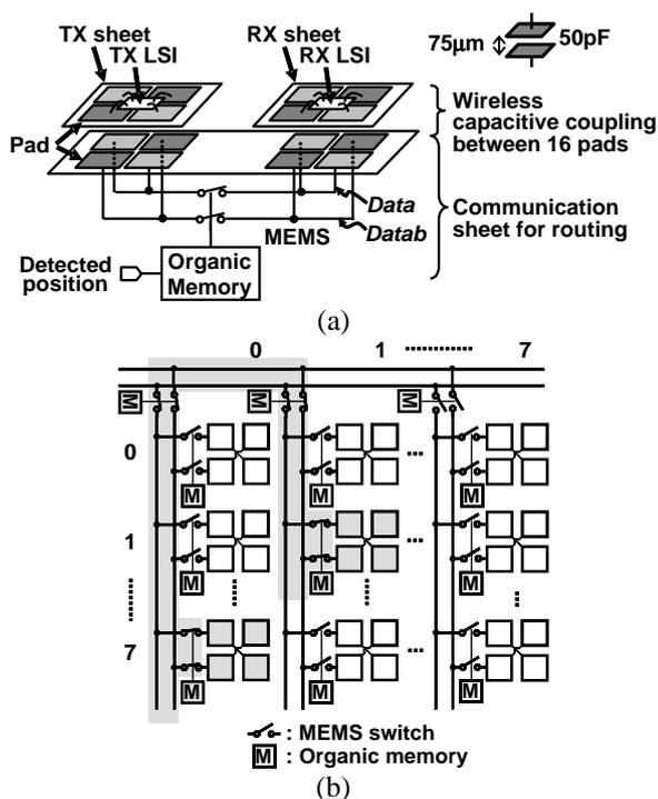
Fig. 1 (a) Overview of the communication system. (b) Communication route.
