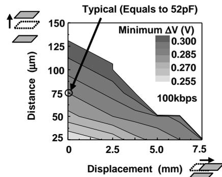
Fig. 4 Measured minimum  $\Delta V$  for different displacement and distance of the pads.
