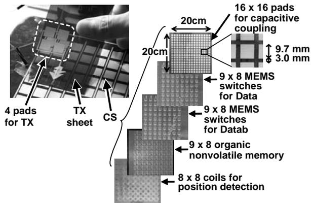
Fig. 2 Device structure of communication sheet.
