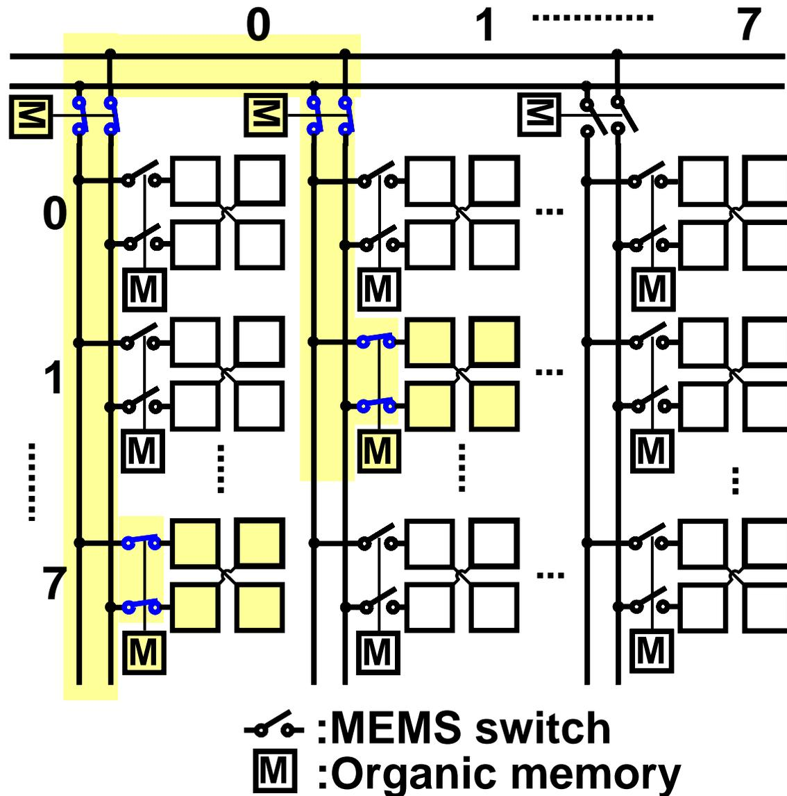
◆ Arbitrary 2 points are connected via 4 switches.
