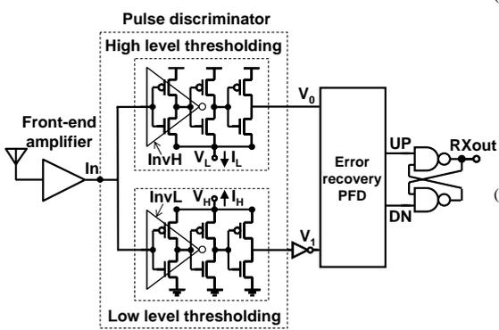
Fig. 3 Proposed RX with DC power-free pulse discriminator.
