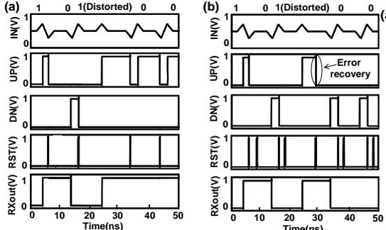
Fig. 6 Simulated waveforms of PFD. (a) Without error-recovery reset. (b) With error-recovery reset.
