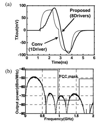
Fig. 2. Simulated TX output. (a) Waveforms. (b) Conv. TX with single driver. (c) Proposed TX with 8 drivers.
