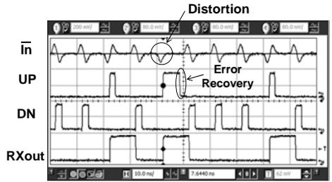
Fig. 9 Measured RX waveforms for distorted data "10100".
