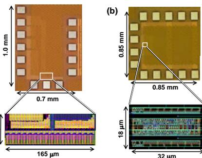
Fig. 7 Chip micrographs and layout. (a) TX. (b) RX.
