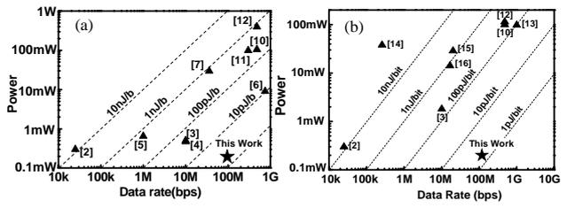
Fig. 11 Comparison with the published UWB transceivers. (a) TX. (b) RX.
