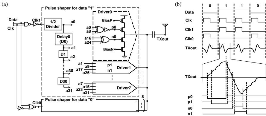
Fig. 1. Proposed digital pulse-shaping TX: (a) Architecture. (b) Timing chart.
