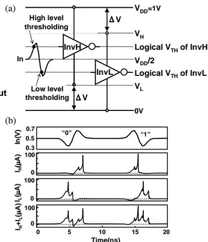
Fig. 4 Pulse discriminator. (a) Operation principle. (b) Simulated waveforms.
