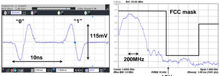
Fig. 8. Measured TX output at 100Mbps. (a) Waveform. (b) Spectrum.
