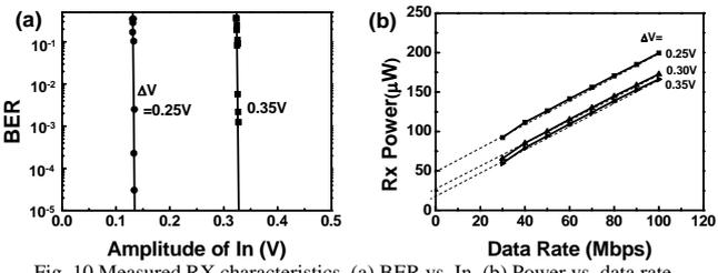
Fig. 10 Measured RX characteristics. (a) BER vs. In. (b) Power vs. data rate.
