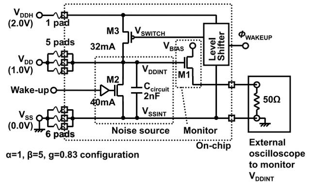
Fig. 7 Schematic of the test chip.
