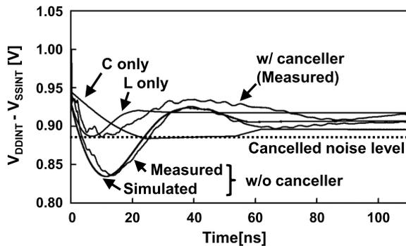
Fig. 17 Noise waveform of passive noise canceller.
