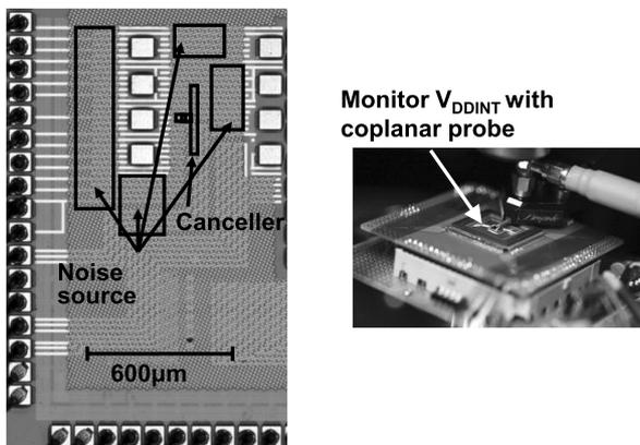
Fig. 10 Chip micrograph and test setup.
