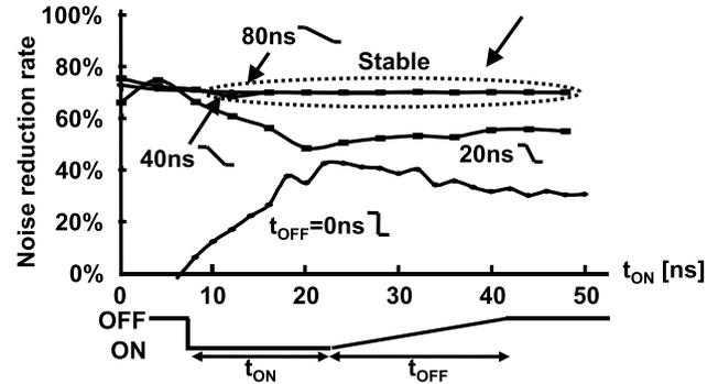
Fig. 14 Turn-off start time vs noise reduction effect.
