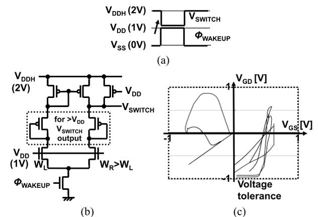
Fig. 8  $V_{SS}$ - $V_{DD}$  to  $V_{DDH}$ - $V_{DD}$  level shifter.
