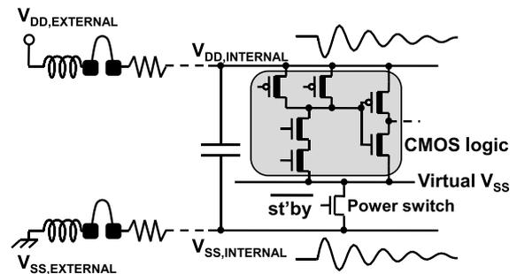
Fig. 1 Power gating and supply line noise.
