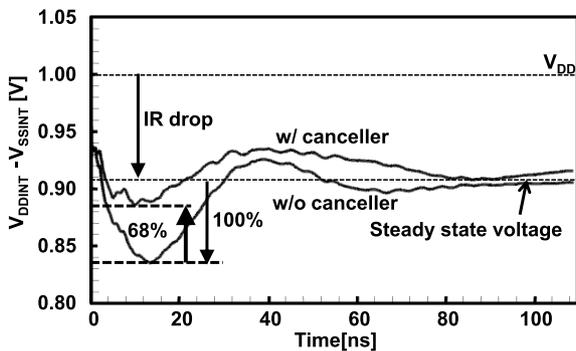
Fig. 9 Measured noise waveform with and without noise canceller.
