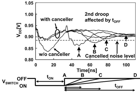
Fig. 12 Measured turn-off time vs noise.
