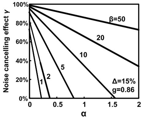
Fig. 6 High voltage factor vs noise cancelling effect.
