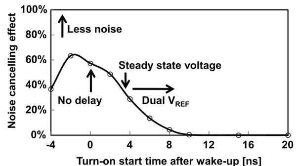
Fig. 11 Turn-on delay vs noise cancelling effect.
