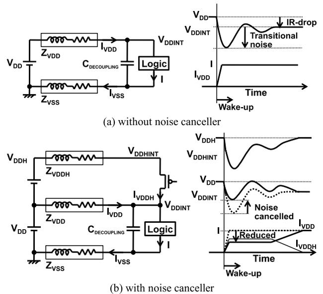
Fig. 5 Configuration and schematic waveform of with and without noise canceller.
