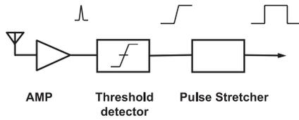
Fig. 5 Block diagram of threshold detection-based UWB receiver.
