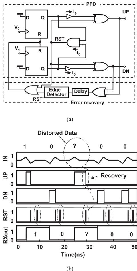
**Fig. 9** Proposed error-recovery phase-frequency detector. (a) Circuit schematics. (b) Error-recovery operation (RXout is shown in Fig. 6).
