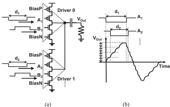
Fig. 2 (a) Proposed UWB pulse generator. (b) Digital pulse-shaping waveforms.
