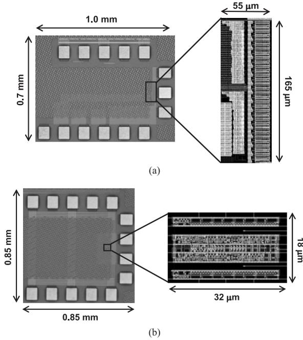
Fig. 10 Chip micrographs and layout. (a) Transmitter. (b) Receiver without front-end amplifier.
