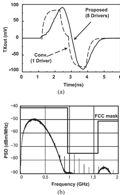
Fig. 4 (a) Waveform comparison between conventional and proposed TX. (b) Modulated transmit spectrum of the proposed TX.
