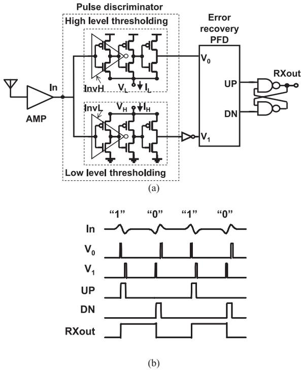
Fig. 6 (a) Circuit schematics of proposed threshold detection-based receiver. (b) Timing chart.
