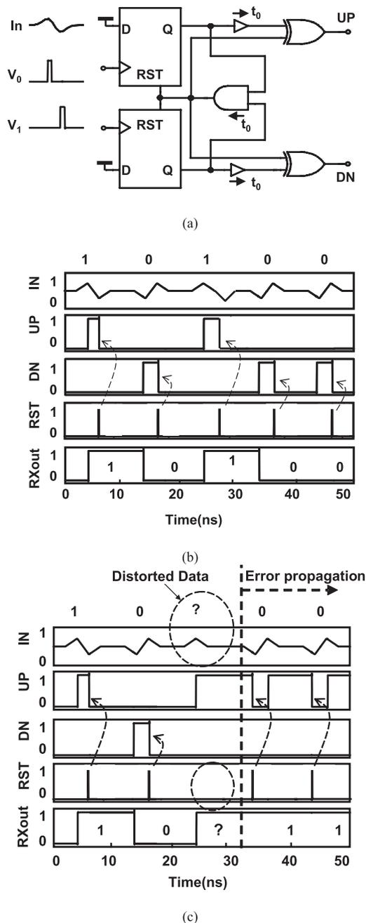
**Fig. 8** Conventional PFD. (a) Circuit schematics. (b) Normal operation (RXout is shown in Fig. 6). (c) Error propagation due to distorted signal.
