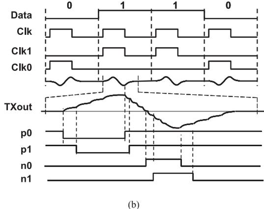
Fig. 3 (a) Overall view of the proposed digital pulse-shaping transmitter. (b) Timing chart.
