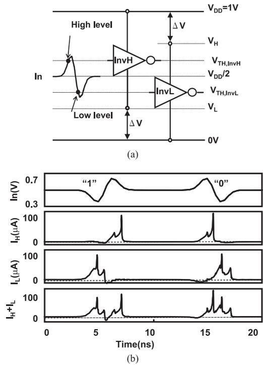
Fig. 7 DC power free pulse discriminator. (a) Operation principle. (b) Simulated waveforms.
