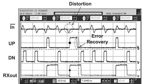
Fig. 12 Measured receiver waveforms for distorted data “10100.”
