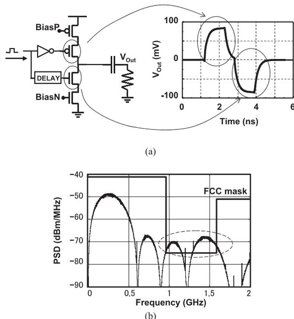
**Fig. 1** (a) Conventional UWB pulse generator. (b) Modulated transmit spectrum.
