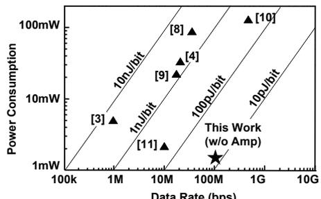
Fig. 9. Comparison with correlation based UWB receivers.
