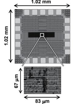
Fig. 6. Micrograph and layout.
