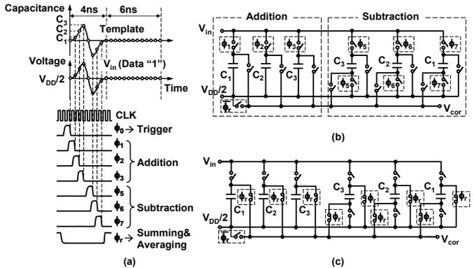
Fig. 3. Charge-domain correlator. (a) Timing chart. (b) Circuit schematics in (b) sampling operation and (c) summing and averaging operation.
