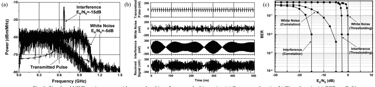
Fig. 1. Simulated UWB environments with narrowband interference and white noise. (a) Frequency domain. (b) Time domain. (c) BER vs.  $E_b/N_0$ .
