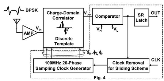
Fig. 2. Impulse UWB receiver with charge-domain correlator and sliding scheme.
