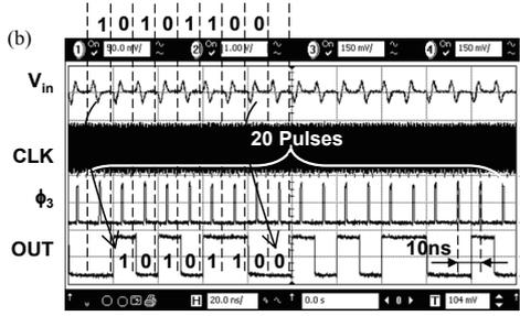
Fig. 7. Measurement results at 100Mb/s. (a) Without sliding scheme. (b) With sliding scheme.
