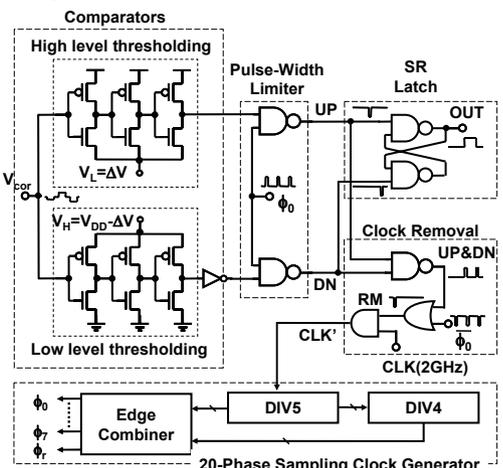
Fig. 4. Circuits for sliding scheme.
