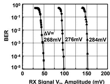
Fig. 8. Measurement results. (a) Power vs. data rate. (b) BER vs. amplitude of  $V_{in}$ . ( $\Delta V$  is defined in Fig. 4.)
