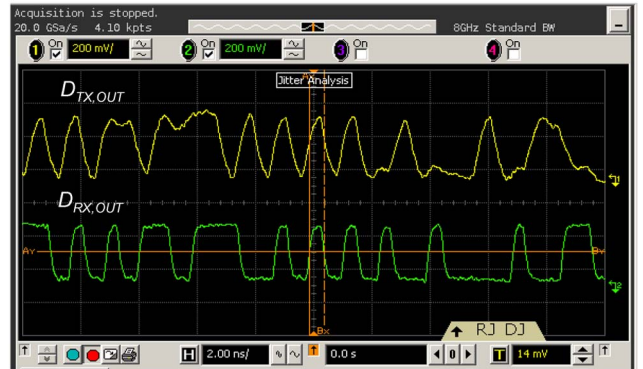
Fig. 7. (a) Test environment. (b) Measured waveforms at the maximum data rate of 2 Gb/s.
