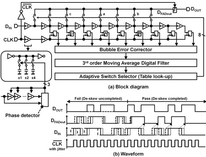
Figure 7.6.3: Feed-forward All-digital De-skewer.
