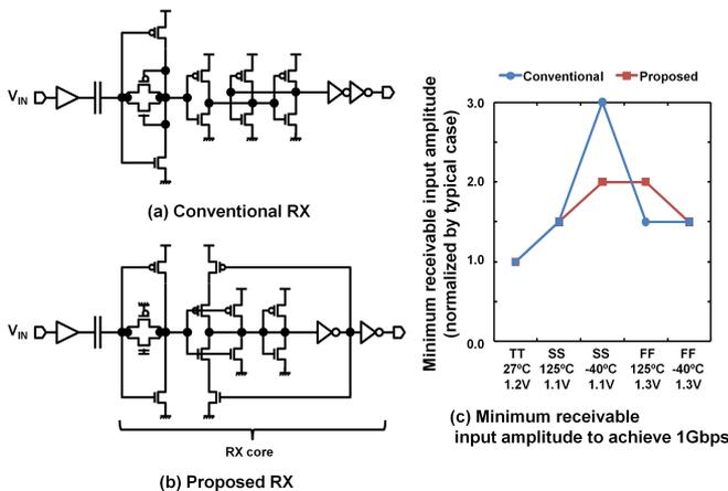
Figure 7.6.5: Comparison of Proposed RX with Conventional RX.
