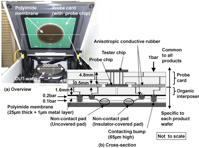
Figure 7.6.1: Wafer-level simultaneous testing scheme.
