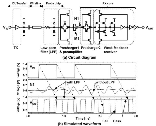
Figure 7.6.4: Proposed RX for a Probe chip.
