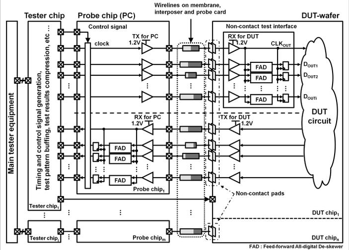
Figure 7.6.2: System block diagram of the proposed WLST system.
