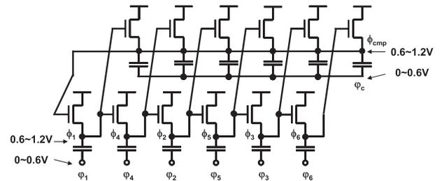
**Fig. 7** Complete circuit schematic of the proposed voltage shifter for both the sampling correlator and the clocked comparator. (© 2010 IEEE)
