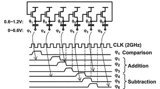
Fig. 5 Simplified circuit schematic of the proposed voltage shifter for the sampling correlator (© 2010 IEEE).
