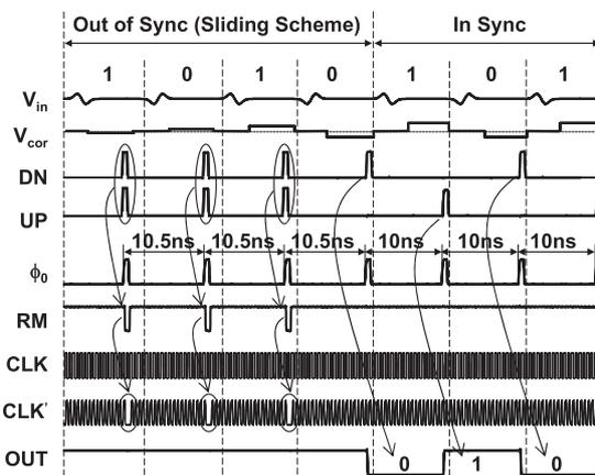
**Fig. 10** Timing chart of sliding scheme for data synchronization.
