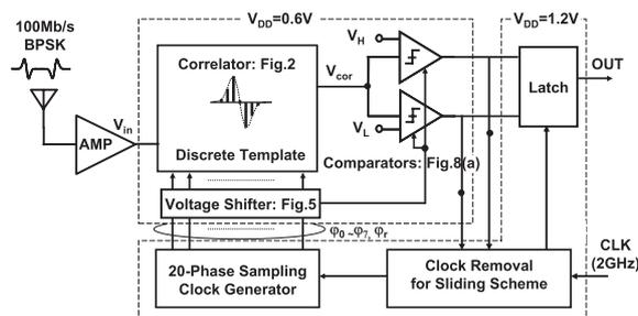
**Fig. 1** Block diagram of impulse radio UWB receiver. 0.6-V voltage shifter supplies boosted voltage to charge-domain correlator and comparator.
