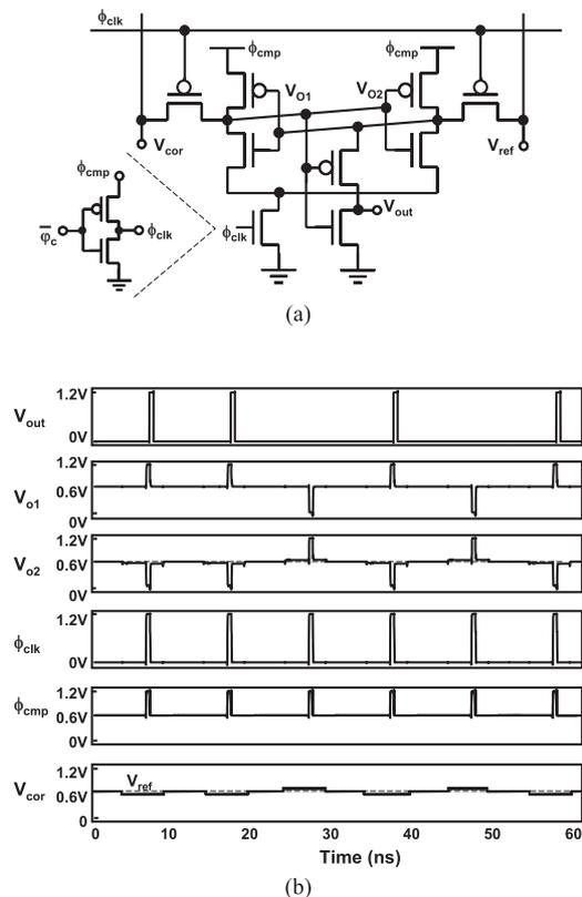
**Fig. 8** Proposed clocked comparator. (a) Circuit schematic. (b) Waveforms. (© 2010 IEEE)
