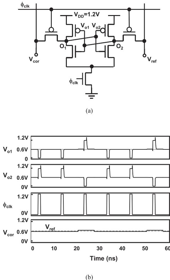
**Fig. 6** Conventional clocked comparator [7]. (a) Circuit schematic. (b) Waveforms. (© 2010 IEEE)
