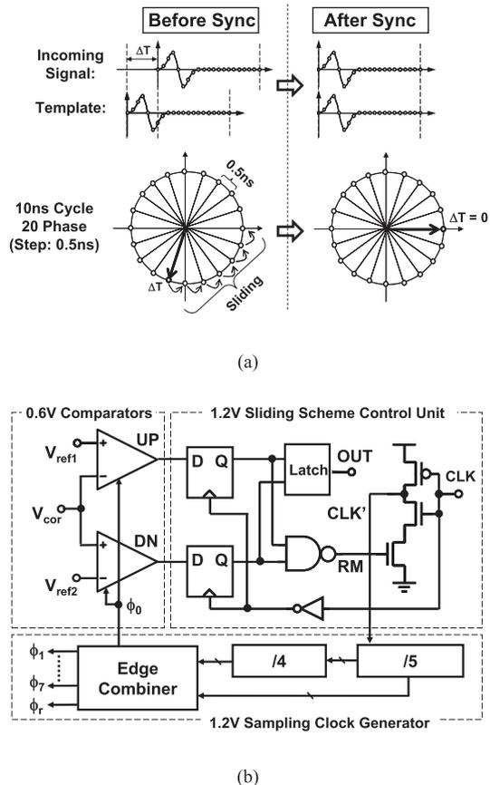
**Fig. 9** Sliding scheme for data synchronization. (a) Operation principle. (b) Circuit implementation.
