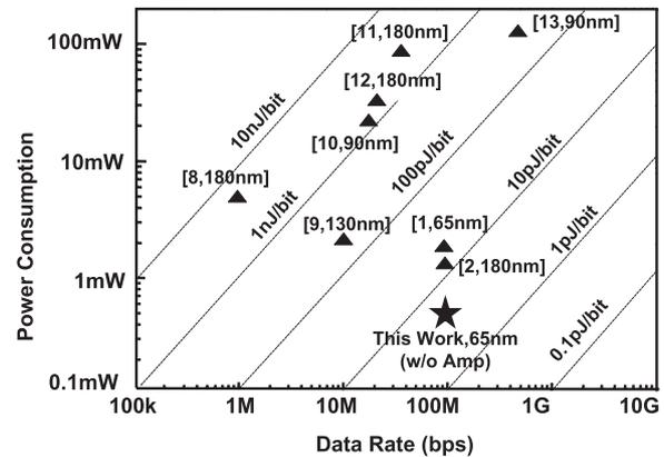
Fig. 13 Comparison with state-of-the-art correlation-based UWB receivers. (Reference and CMOS process technology are shown. [1], [2] are without front-end amp. [8]–[13] are with front-end amp.)
