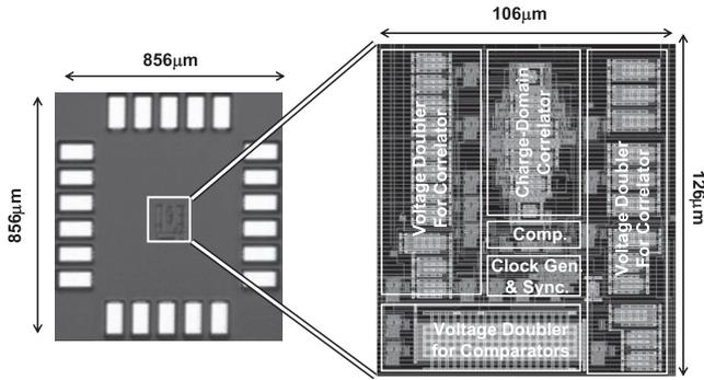
Fig. 11 Chip micrograph and layout of UWB receiver. (© 2010 IEEE)
