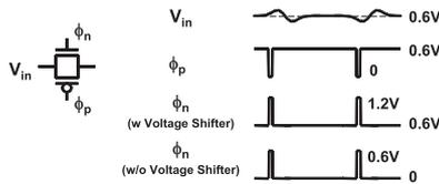
Fig. 3 Split swing level scheme for CMOS transmission gate.
