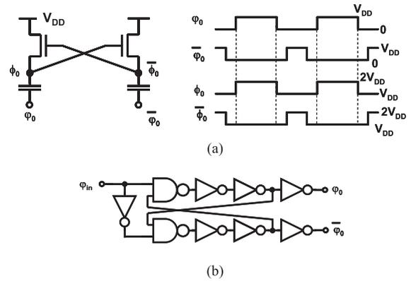
Fig. 4 Conventional voltage shifter [6]. (a) Circuit schematic and waveforms. (b) Non-overlapping complementary clock generator (© 2010 IEEE).
