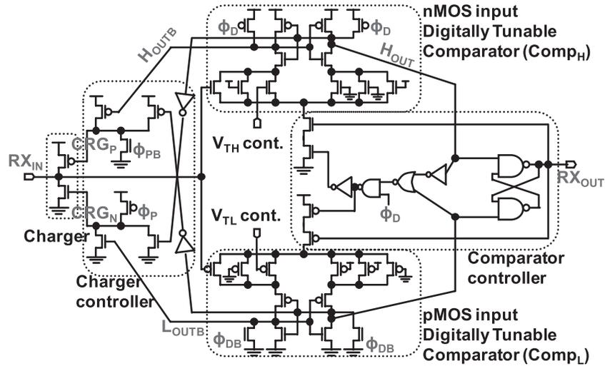
Fig. 3 Receiver circuit schematic of contact allowing wireless connector.
