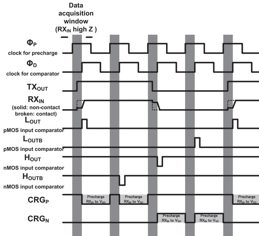
Fig. 4 Detailed timing charts of wireless connector.
