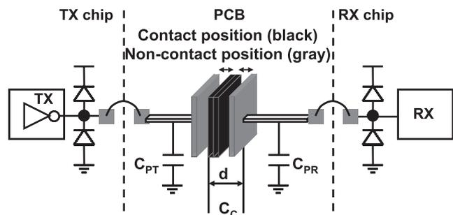
**Fig. 2** A generic capacitive coupling connector circuit.
