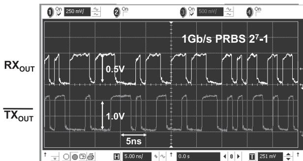
Fig. 8 Measured waveforms of input and output at 1 Gb/s.
