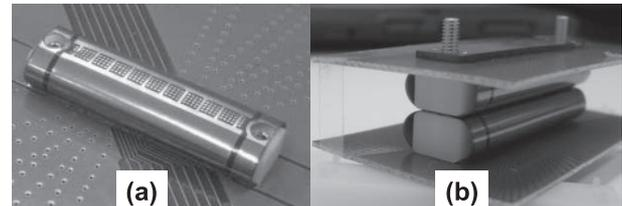
**Fig. 1** Examples of wireless connectors (a) showing capacitive coupling pads and (b) in closed circuit configuration. (Structure applicable but not used in this work)
