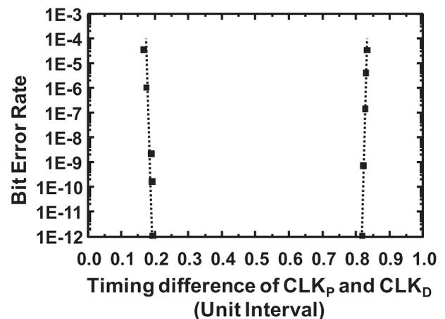
Fig. 10 Measured BER at 800 Mb/s showing a 750 ps timing margin between  $CLK_P$  and  $CLK_D$ , and stable communication.
