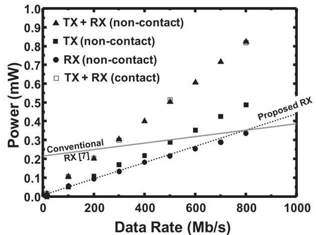
Fig. 9 Power dissipation of TX and RX circuits when contacting and not contacting.
