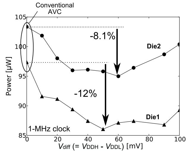
Fig. 8. Measured dependence of power consumption on  $V_{diff}$ .
