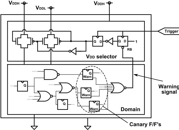
Fig. 3. Circuit schematic of each domain in FADVC.
