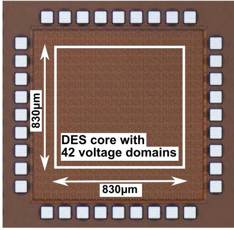
Fig. 6. Microphotograph of test chip in 40-nm CMOS process including a DES core divided into  $6 \times 7$  voltage domains.
