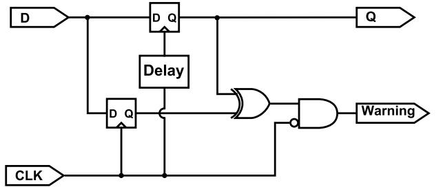
Fig. 4. Circuit schematic of canary F/F.
