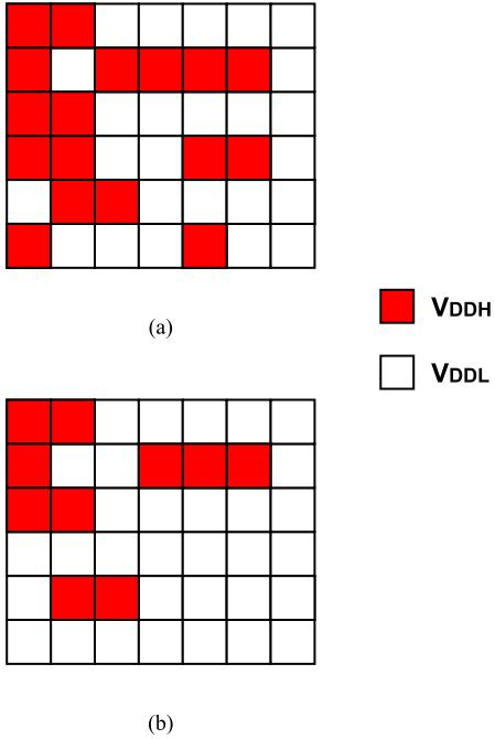
Fig. 9. Measured distributions of  $V_{DDH}$  and  $V_{DDL}$  among 42 voltage domains at minimum power conditions of (a) die1 and (b) die2.
