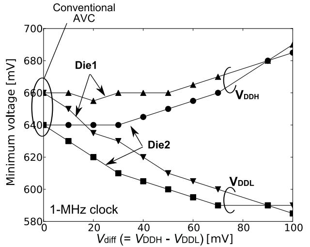
Fig. 7. Measured dependence of minimum supply voltage on  $V_{diff}$ .
