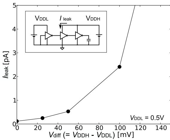
Fig. 10. Simulated dependence of leakage current between two domains with  $V_{diff}$  difference.
