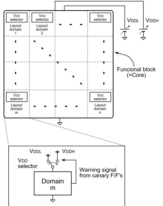
Fig. 2. Proposed within-functional-block fine-grained adaptive dual supply voltage control (FADVC)
