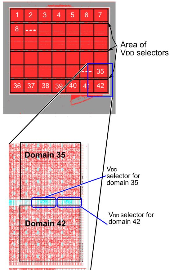
Fig. 5. Layout of fabricated test chip. DES core is divided into  $6 \times 7$  voltage domains.
