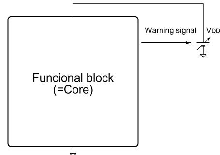
Fig. 1. Conventional adaptive voltage control (AVC).
