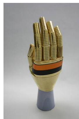
Fig. 1. Implementation example of electronic artificial skin (E-skin), which is sheet containing array of pressure sensors and OFETs.
