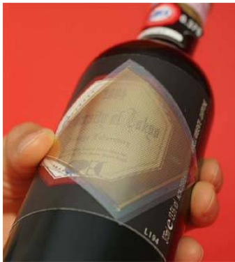
Fig. 3. Sheet-type image scanner, which is sheet integrating array of photodetectors and OFETs.
