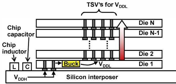
Fig. 7. Conventional power supply scheme.
