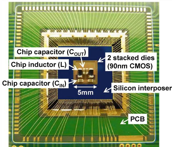
Fig. 11. Photograph of assembled system on a PCB board. Chip inductor and chip capacitor are mounted directly on top of stacked dies at the center of the photo.
