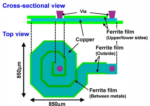
Fig. 3. Layout of spiral ferrite inductor.
