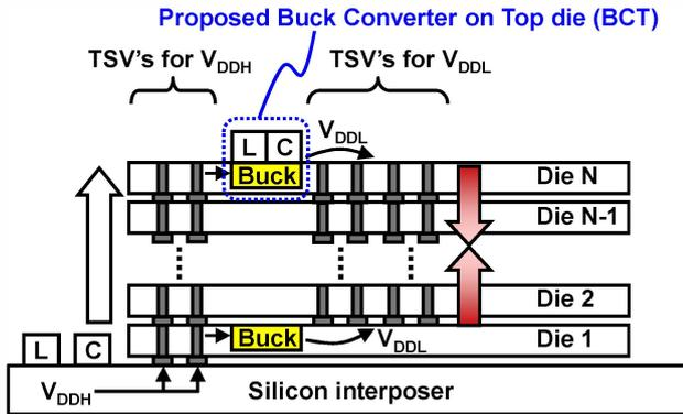
Fig. 8. Proposed Buck Converter on Top die (BCT) scheme.
