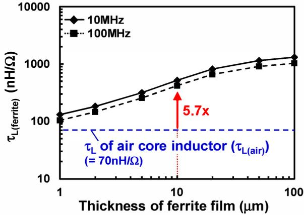
Fig. 4. Dependence of  $\tau_L$  of ferrite inductor and air core inductor.
