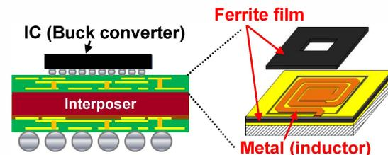
Fig. 1. Inductor on Interposer with ferrite film.
