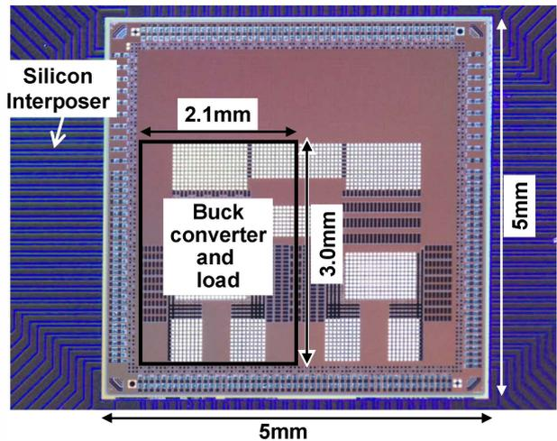
Fig. 10. Two stacked dies using TSV's are mounted on top of a silicon interposer.
