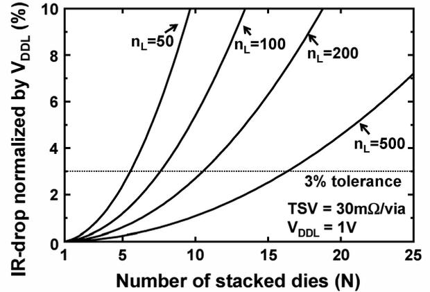
Fig. 6. Calculated IR drop in 3D integration.  $n_L$  is the total number of TSV's per die used for power delivery. Each die is assumed to consume 1A.
