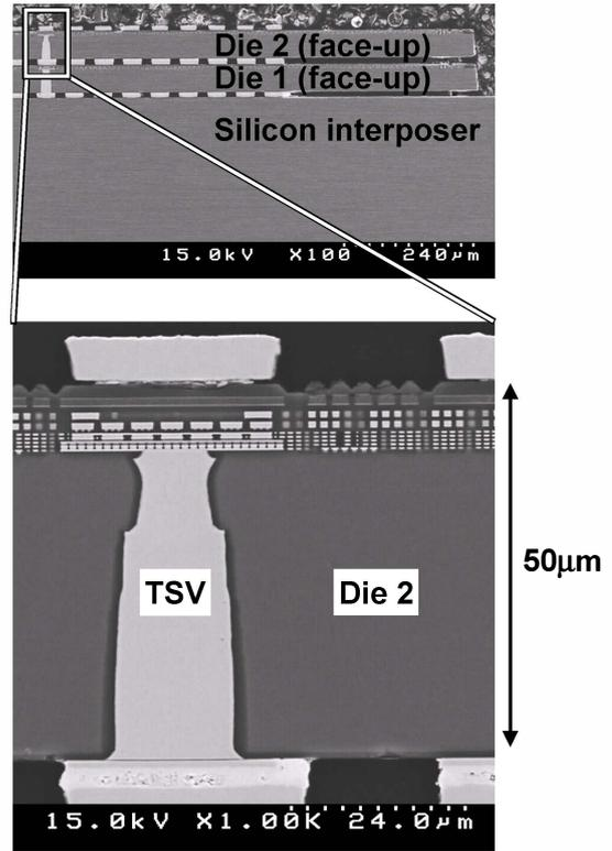
Fig. 9. Cross sectional view of 3D integrated system. The upper photo is a global view and the lower photo is a magnified view around a TSV.
