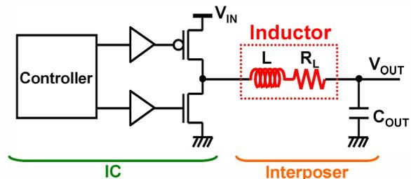
Fig. 2. Circuit schematic of buck converter with inductor on interposer.
