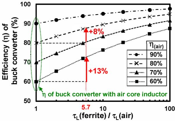
Fig. 5. Efficiency increase of buck converter by using ferrite inductor.
