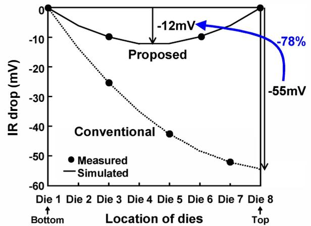
Fig. 12. Measured IR drop and simulated results.
