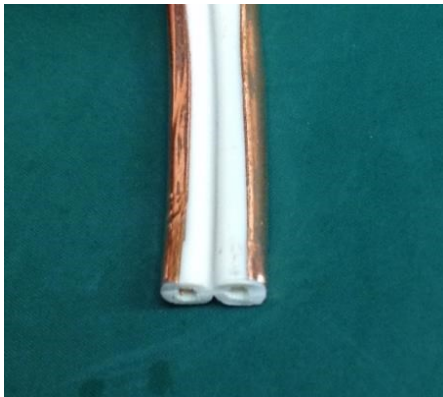
Fig. 2. Photo of the two-wire power cords with the two electrodes for EHICPC.
