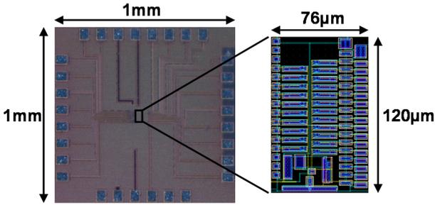
Fig. 7. Die photo and layout of proposed glitch-free programmable voltage detector in 250-nm CMOS.
