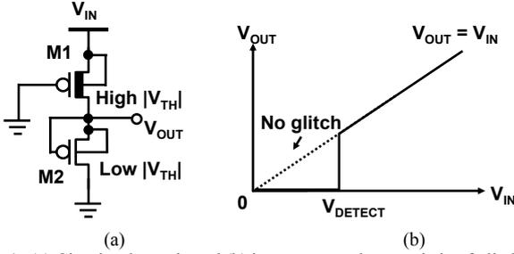
Fig. 4. (a) Circuit schematic and (b) input-output characteristic of glitch-free voltage detector.
