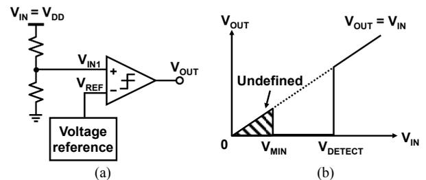
Fig. 2. (a) Circuit schematic and (b) input-output characteristic of commercially available voltage detector [5-7].
