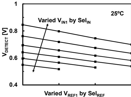
Fig. 10. Measured programmable  $V_{DETECT}$  in proposed glitch-free programmable voltage detector.
