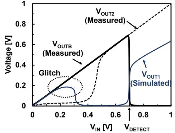
Fig. 8. Simulated and measured input-output characteristics of proposed glitch-free programmable voltage detector.
