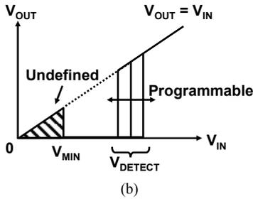
Fig. 3. (a) Circuit schematic and (b) input-output characteristic of conventional programmable voltage detector.
