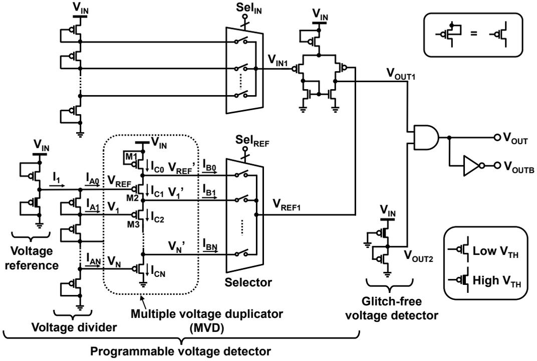
Fig. 6. Circuit schematic of proposed glitch-free programmable voltage detector.
