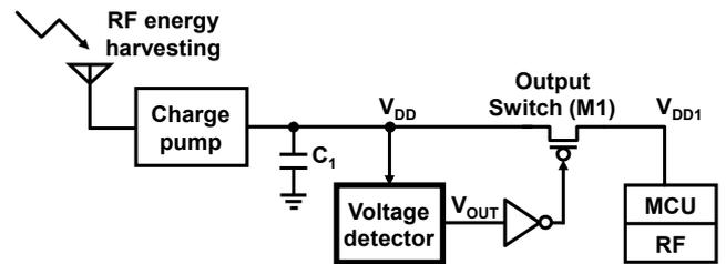
Fig. 1. Block diagram of IoT node with RF energy harvesting.
