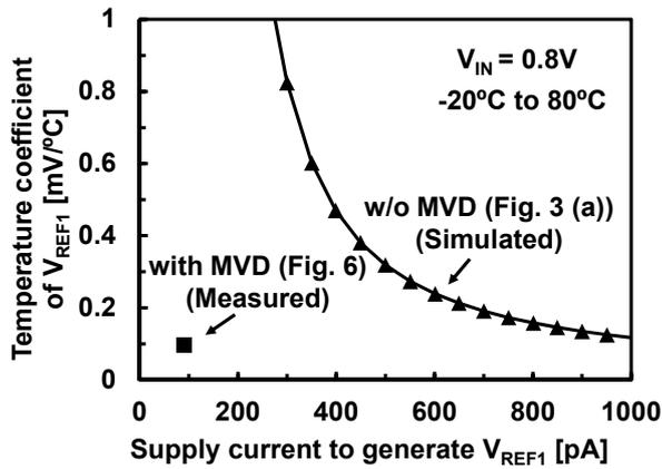
Fig. 9. Power supply current dependence of temperature coefficient of  $V_{REF1}$  with and without proposed multiple voltage duplicator (MVD).
