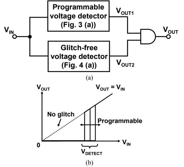
Fig. 5. (a) Block diagram and (b) input-output characteristic of proposed glitch-free programmable voltage detector.
