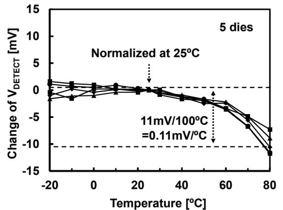
Fig. 11. Measured temperature dependence of  $V_{DETECT}$  among 5 dies of proposed glitch-free programmable voltage detector.
