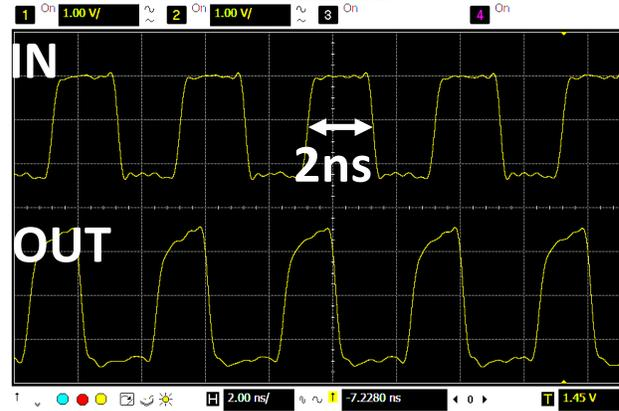
Fig. 9. Measured 500Mbps operation
