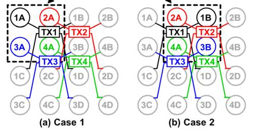
Fig. 5. Proposed 4 × 4 alternate TX coil array.
