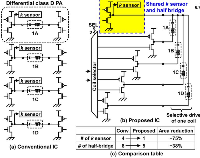
Fig. 4. Proposed shared topology in AMFA IC.
