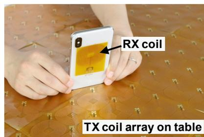
Fig. 1. Application scenario of perpendicular WPT.
