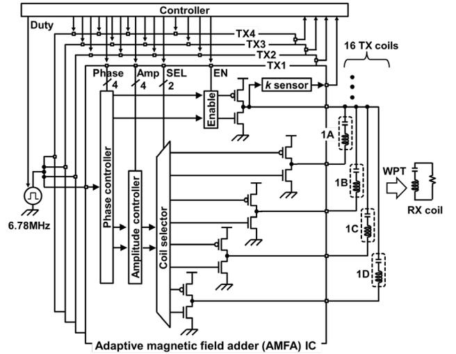
Fig. 3. Block diagram of 6.78 MHz wireless power transfer system.
