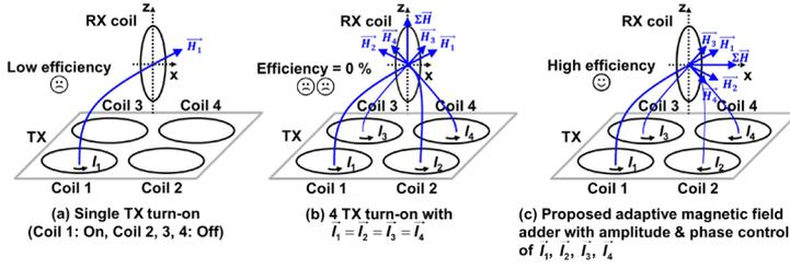
Fig. 2. Three control methods for perpendicular WPT.
