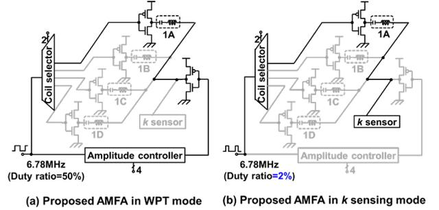
Fig. 6. Two modes of AMFA IC. (a) WPT mode. (b) k sensing mode.
