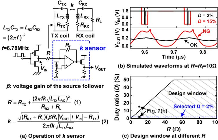
Fig. 7. Operating principle of proposed k sensor.
