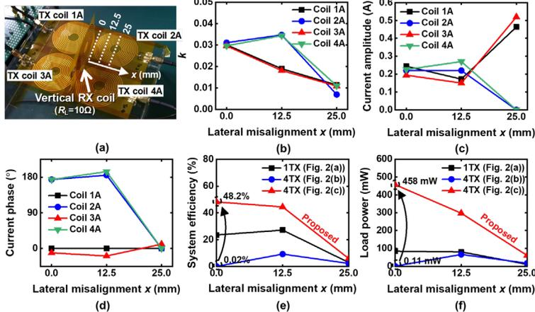
Fig. 10. (a) Measurement setup corresponding to Fig. 5(a). (b)-(f) Measurement results of wireless power transfer system.
